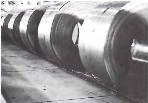
Hot Rolled Coil Conveyor
